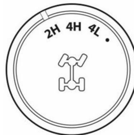
4L All-wheel drive and low gear range 2.542 transfer case low gear ratio is ideally suited for driving on the worst rugged terrains
